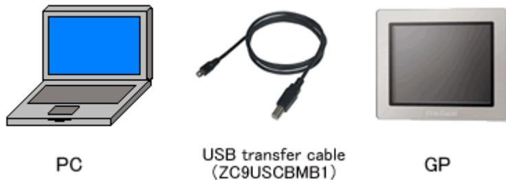
1. Connect your PC and GP-4201TM with a USB transfer cable (model: ZC9USCBMB1). If the driver of the cable has not been installed on your PC yet, a dialog box will appear. Please follow the instructions.
