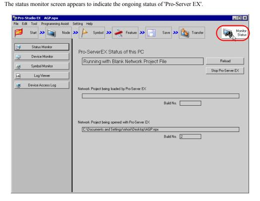
• To perform device monitoring, 'Pro-Server EX' should be operating. When 'Pro-Server EX' is under suspension, click the [Reload] button to start the operation.
