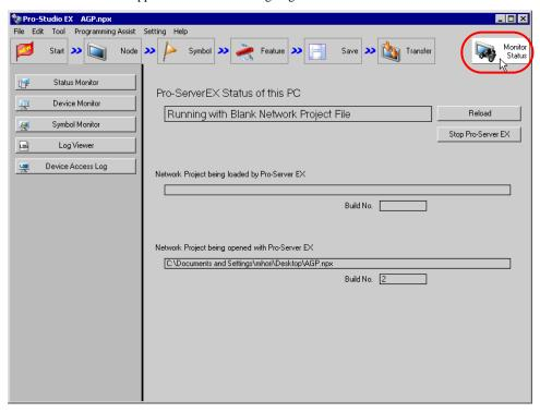
• To perform symbol monitoring, 'Pro-Server EX' should be operating. When 'Pro-Server EX' is under suspension, click the [Reload] button to start the operation.
