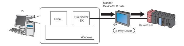
(2) The 'Pro-Server EX' notifies 'Excel' of a change in the data in the Device/PLC, if any.
