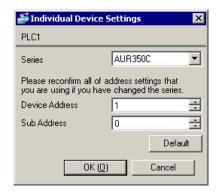
To configure communication settings for the External Device, use the ADDRESS switch on the External Device and the setting tool (Smart Loader Package SLP-A35).
