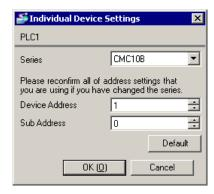
Use the ladder software (Smart Loader Package SLP-CM1 V2.0.1) to configure communication settings for the External Device. Use the rotary switch on the front of the Controller to set the device address and transmission speed of the External Device.
