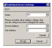
To configure communication settings for the External Device, use the setting tool (Smart Loader Package SLP-RXE).
