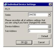
Use the ladder software (Smart Loader Package SLP-D510 V2.2.3) to configure communication settings for the External Device. Use the rotary switch on the front of the Controller to set the device address of the External Device.
