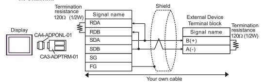
1:n Connection Shield Termination resistance Signal name External Device External Device 120Ω (1/2W) RDA Terminal block Terminal block Shield Termination resistance Display RDB Signal name Signal name 120Ω (1/2W) CA4-ADPONL-01 SDA B(+) B(+) SDB A(-) A(-) CA3-ADPTRM-01 SG FG Your own cable
