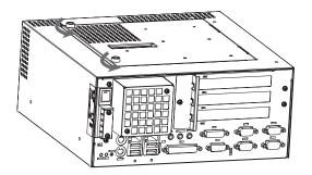
1) Loosen the two (2) maintenance cover attachment screws.
