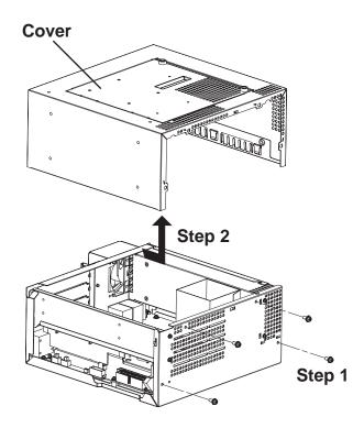
1) Lay the PS-B unit on its side and unscrew the four (4) cover attachment screws.
