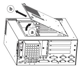
2) Tilt the maintenance cover up as shown by arrow a and lift it out in the direction shown by arrow b (see diagram).
