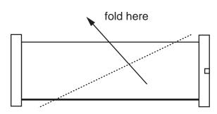
4) As shown in the left-side figure, fold the cable over, along the dotted line.
