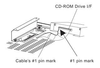
4) Connect the PSS-CD01 to the PS-A unit via the connection cable. Be sure to that the Cable's #1 pin mark and the connector are correctly aligned.
