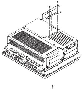
2) Secure PL fastener (C) to the rear of the PL unit using the two (2) attachment screws.
