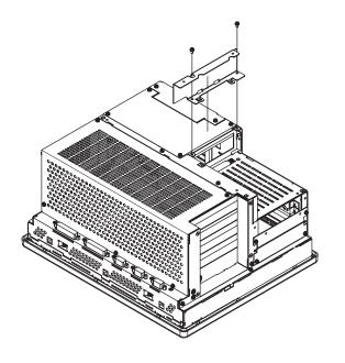
2) Secure PL fastener (C) to the rear of the PL unit using the two (2) attachment screws.
