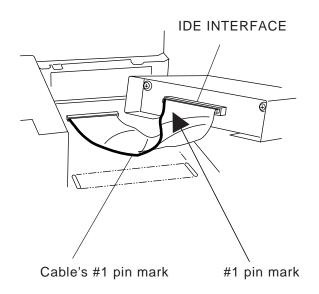
5) Connect the PSS-CD01 unit to the PL unit via the connection cable. Be sure to confirm that the Cable's #1 pin mark and the connector are correctly aligned.
