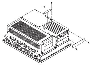
1) Unscrew the IDE I/F cover's two (2) attachment screws and the HDD1 slot's two (2) attachment screws. Remove the IDE I/F cover and the HDD1 slot cover.
