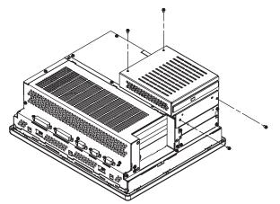
6) Secure the PSS-CD01 unit to the PL unit using the four (4) attachment screws. Place the cable in the space between the PSS-CD01 and the PL unit.
