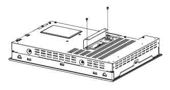
2) Secure PS-A fastener (A) to the rear of the PS-A unit using the two (2) attachment screws. Fastening torque should be 0.5 to 0.6N•m.
