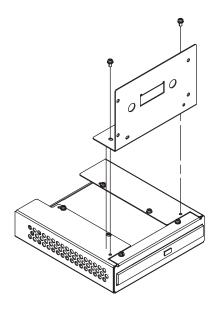
3) Secure PL fastener (D) to the PSS-CD01 unit using the two (2) attachment screws.
