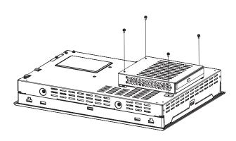
5) Secure the PSS-CD01 to the PS-A unit using the four (4) attachment screws. Fastening torque should be 0.5 to 0.6N•m. Place the cable in the space between the PSS-CD01 and the PS-A unit.
