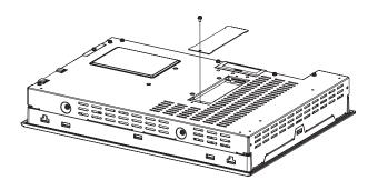
1) Unscrew the CD-ROM Drive I/F cover's attachment screw and remove the CD-ROM Drive I/F cover.
