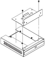
3) Secure PL fastener (D) to the PSS-CD01 unit using the two (2) attachment screws.
