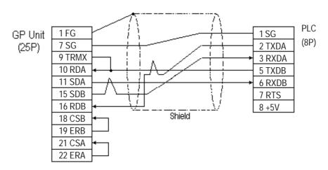
Note: Connecting #9 and #10 pins in the GP Serial I/F adds a termination resistance of  $100\Omega$  between RDA and RDB.
