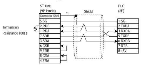
\*1 Be sure to connect the shield to the Connector Shell. For information about FG connections, refer to page 1-2 "RS422 I/F (ST400)" section's Note, in the "Connecting a Device/PLC to the ST unit."
