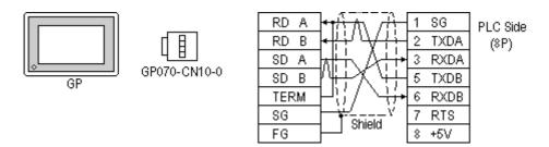
• When using Digital's RS-422 cable, GP230-IS11-0
