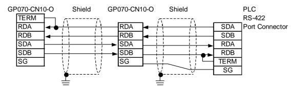
• When using Digital's Multi-link Cable, GP230-IS12-O
