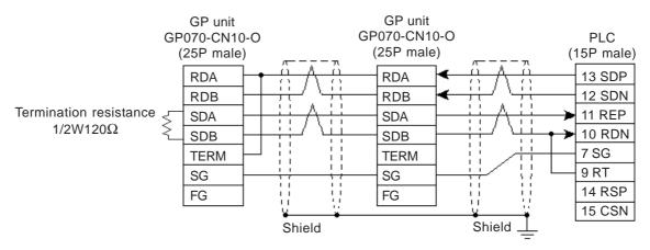
• When using Digital's Multi-link Cable, GP230-IS12-O
