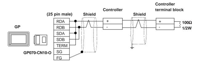
• Using Digital's RS-422 cable, GP230-IS11-0
