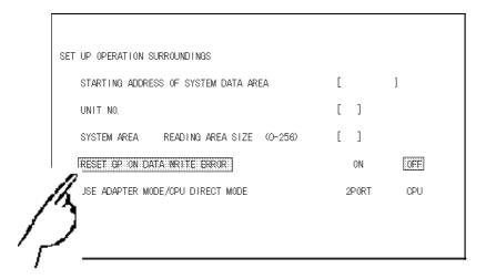
4) Touch the "RESET GP ON DATA WRITE ERROR" selection. The selected item is highlighted.
