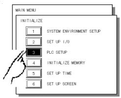
2) Touch item #3, PLC SETUP. The PLC SETUP menu appears.
