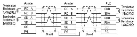
• When using Digital's Multi-link Cable, GP230-IS12-O
