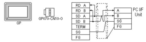
• When using Digital's RS-422 Cable, GP230-IS11-0
