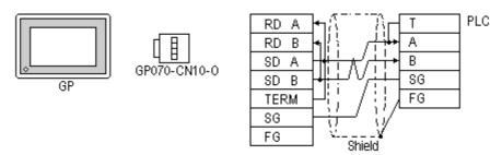
• When using Digital's RS-422 Cable, GP230-IS11-0
