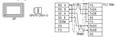
• When using Digital's RS-422 Cable, GP230-IS11-0
