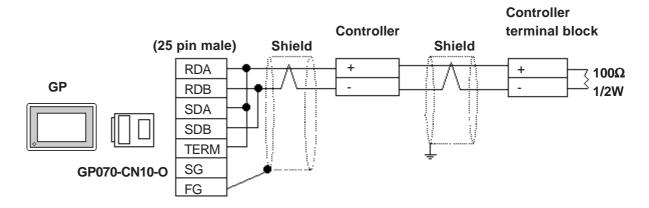
• Using Digital's RS-422 cable, GP230-IS11-0
