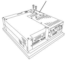
3) Unscrew the two rear face Blank Panel attachment screws, and remove the Blank Panel.
