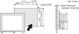
(2) Confirm that the installation gasket is attached to the PL unit and then place the PL unit into the Panel from the front.
