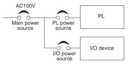
Wire the power cords of the PL, I/O devices, and power supply devices separately.
