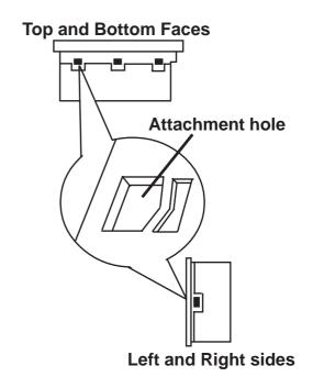
4) Slowly tighten each fastener attachment screw in sequence (top, bottom, left side, right side), until all fastener are evenly and securely tightened.
