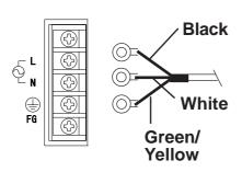
2) Loosen and remove the middle three (3) screws from the terminal strip. Align the crimp terminals with each screw hole, and tighten the screws.
