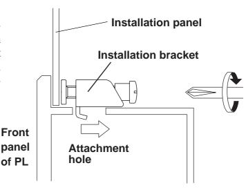
Excessive torque may damage the panel or bracket. To ensure a high Important degree of moisture resistance, the torque should be 0.5 Nom.
