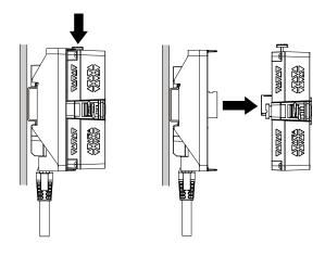
2. Push down on the rear module installation adapter and unhook the bottom part of the adapter from the DIN rail.
