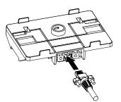
2. Position the top groove of the rear module installation adapter on the top edge of the DIN rail.
