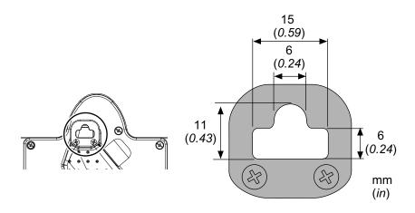
The wall and wall hanging bracket must be able to withstand loads of 20 kg (44.1 lb) or more.
