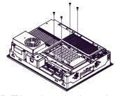
(7) With opposite procedure above, set the DISK cover, expansion board base, and expansion board cover to the PS-A unit, respectively. The torque required to tighten these screws is 0.5 to 0.6 N·m.
