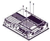
(5) With opposite procedure above, set the DISK cover to the PS-A unit. The torque required to tighten these screws is 0.5 to 0.6 N·m.
