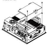
(3) Unscrew the expansion board base's screws (4) and remove the expansion board base
