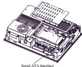
(5) Mount the HDD unit vertically on the circuit board and plug the HDD unit cable connector in the Serial ATA interface.
