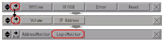
**3** When the [LogicMonitor] switch is touched, the following screen appears. You can check whether the transferred logic program is operating properly.
