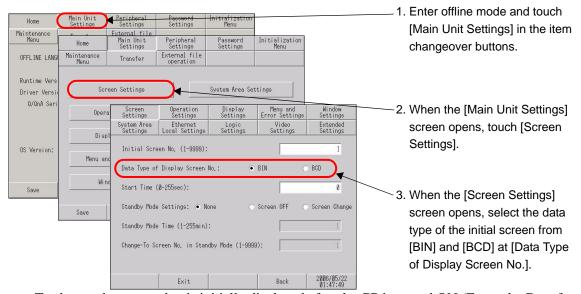
To change the screen that is initially displayed after the GP is turned ON (Example: Data format of the screen No. is BIN, Base screen 10), adjust the settings as follows:
