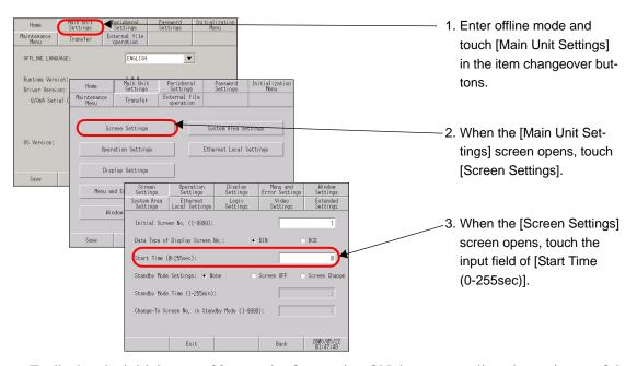
To display the initial screen 30 seconds after turning ON the power, adjust the settings as follows:
