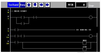
4 To exit Logic Monitor, touch [Toolband] and then touch in the toolband. Touch [QUIT] to return to the RUN screen.
