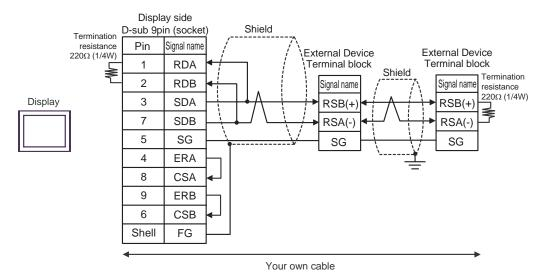
C) When using the online adapter (CA4-ADPONL-01) by Pro-face, the terminal block conversion adapter (CA3-ADPTRM-01) by Pro-face and your own cable
