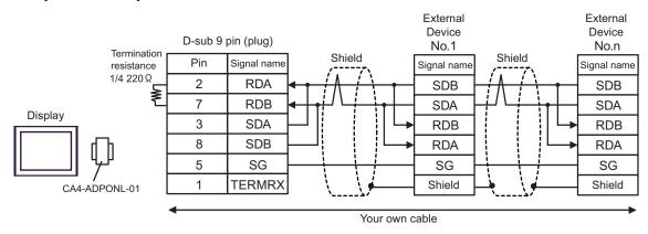
E) When using the COM port conversion adapter (CA3-ADPCOM-01), the terminal block conversion adapter (CA3-ADPTRM-01) by Pro-face and your own cable
