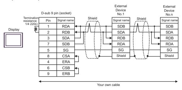
C) When using the online adapter (CA4-ADPONL-01) by Pro-face, the terminal block conversion adapter (CA3-ADPTRM-01) by Pro-face and your own cable
