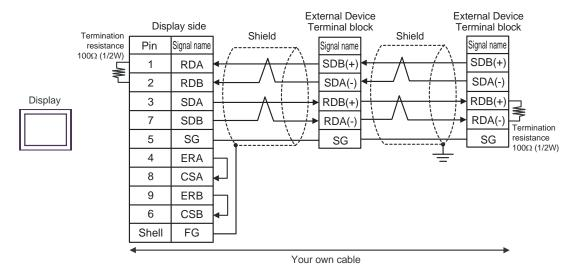
C) When using the online adapter (CA4-ADPONL-01) by Pro-face, the terminal block conversion adapter (CA3-ADPTRM-01) by Pro-face and your own cable
