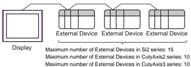
• 1:n Connection (when using both COM1 and COM2)
