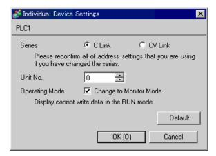
Set the HOST link unit attached to the External Device as below.
