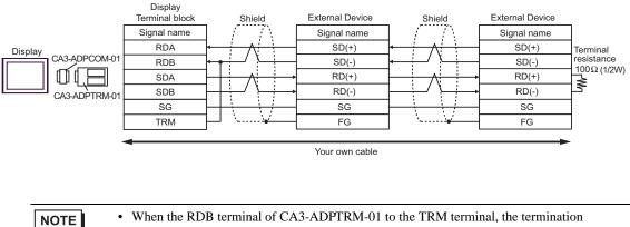
resistance of  $100\Omega$  (1/2W) is inserted between RDA and RDB terminals on the Display.
