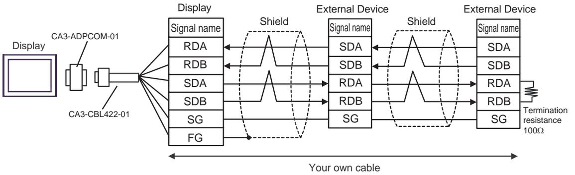
C) When using the RS-422 cable (CA3-CBL422/5M-01) by Pro-face and your own cable
