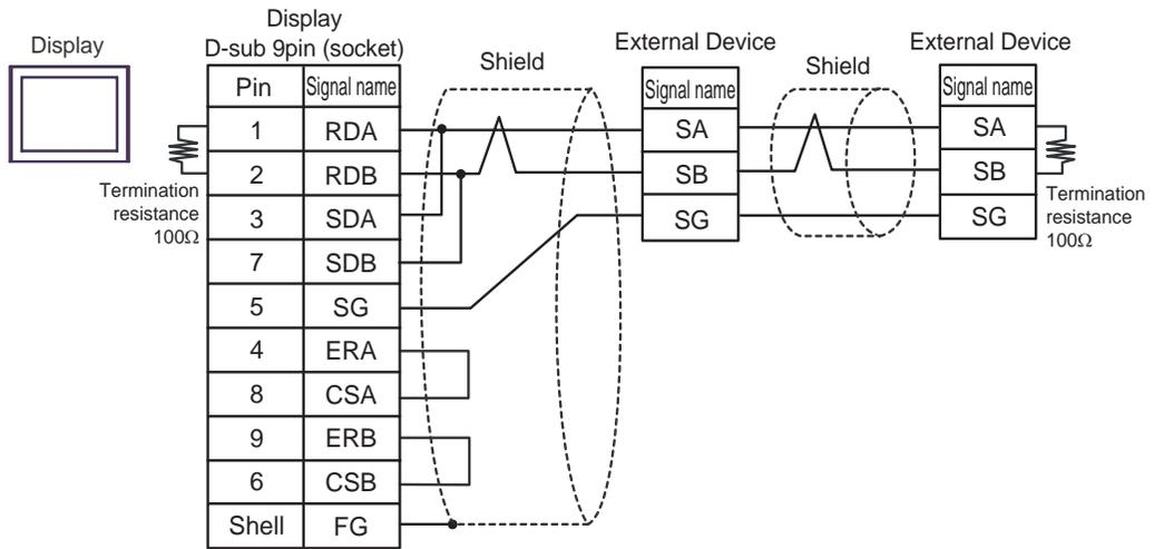
C) When using the online adapter (CA4-ADPONL-01), the terminal block conversion adapter (CA3-ADPTRM-01) by Pro-face and your own cable
