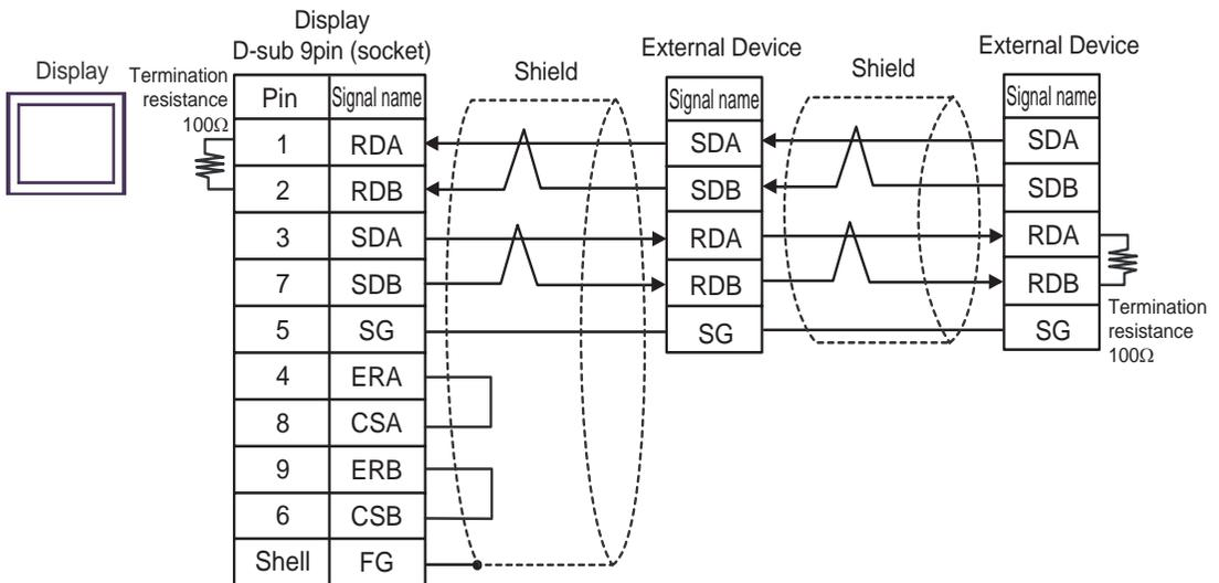
E) When using the online adapter (CA4-ADPONL-01), the terminal block conversion adapter (CA3-ADPTRM-01) by Pro-face and your own cable
