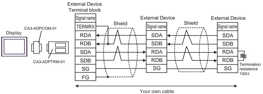
B) When using the COM port conversion adapter (CA3-ADPCOM-01), the RS-422 cable (CA3-CBL422-01) by Pro-face and your own cable
