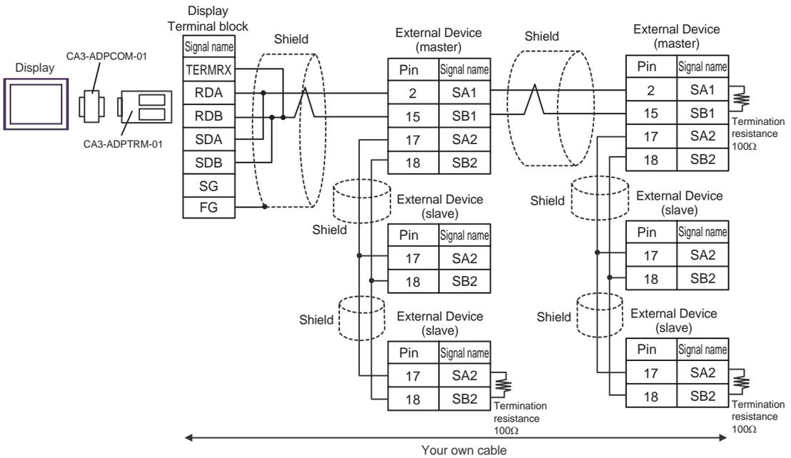
**IMPORTANT** • Connect No. 17 and No. 18 between slaves as shown in the figure above.
