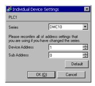
Use the ladder software to configure communication settings for the External Device. (Operation confirmed using the the Smart Loader Package SLP-D10 V3.0.1.) Set the device address of the External Device using the rotary switch on the front of the Controller.
