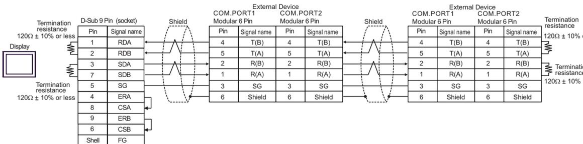
C) When using the online adapter (CA4-ADPONL-01), the terminal block conversion adapter (CA3-ADPTRM-01) by Pro-face
