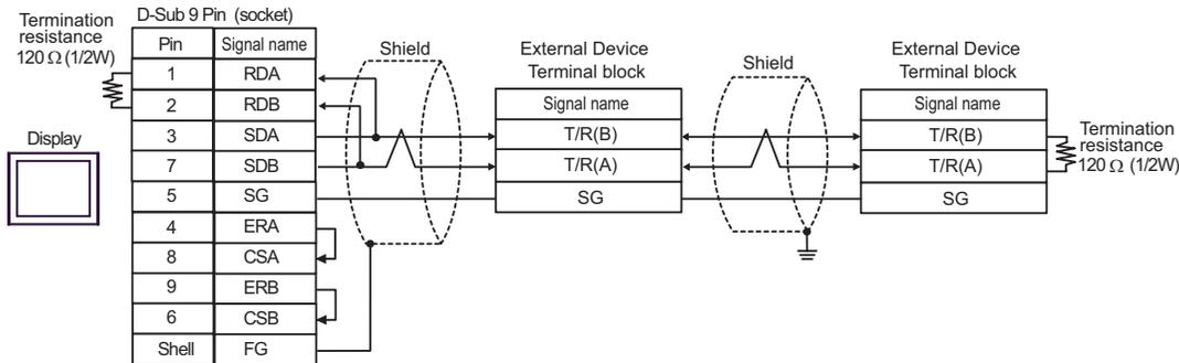
C) When using the online adapter (CA4-ADPONL-01), the terminal block conversion adapter (CA3-ADPTRM-01) by Pro-face
