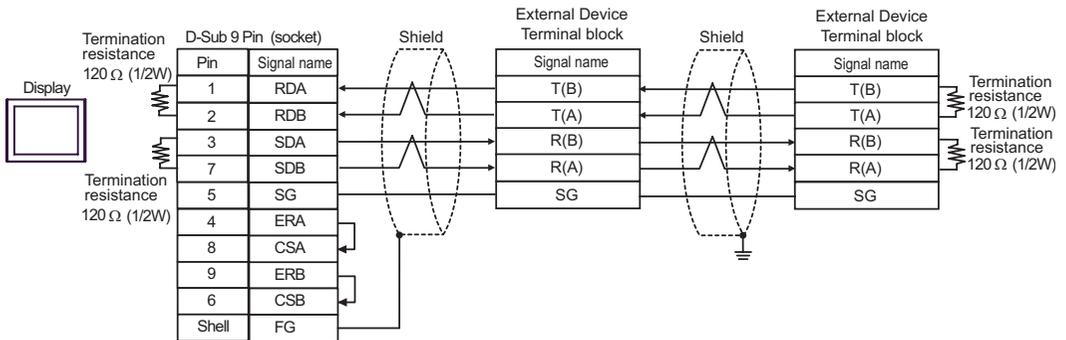
C) When using the online adapter (CA4-ADPONL-01), the terminal block conversion adapter (CA3-ADPTRM-01) by Pro-face
