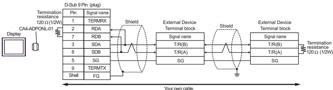
E) When using the COM port conversion adapter (CA3-ADPCOM-01) and the terminal block conversion adapter (CA3-ADPTRM-01) by Pro-face
