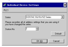
Use the ladder software (DirectSOFT32 programming version 4.0) for communication settings. After completing the settings, reboot the External Device to enable them. Please refer to the manual of the External Device for details.
