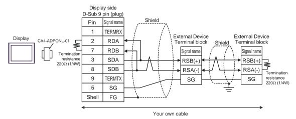
E) When using the COM port conversion adapter (CA3-ADPCOM-01), the terminal block conversion adapter (CA3-ADPTRM-01) by Pro-face and your own cable
