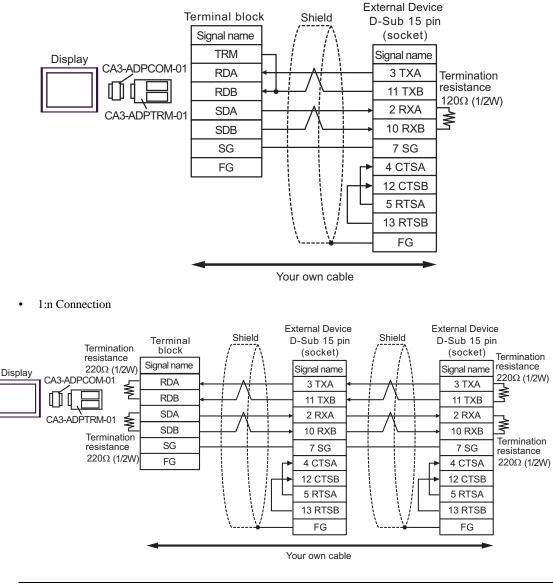
• When IPC is used as the Display, the terminal resistance of  $220\Omega$  can be inserted by the fact that the dip switch 5, 6 of IPC is turned to ON.
