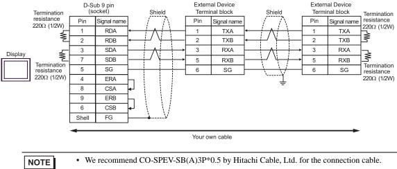
• When IPC is used as the Display, the terminal resistance of  $220\Omega$  can be inserted by the fact that the dip switch 5, 6 of IPC is turned to ON.
