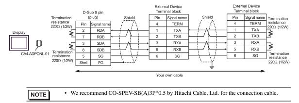
F.When using the online adapter (CA4-ADPONL-01) and the RS422 cable (CA3-CBL422-01) by Digital Electronics Corp.
