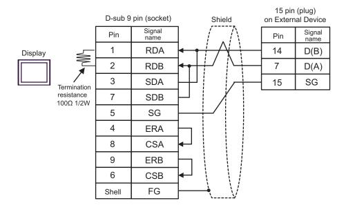
C) When using the online adapter (CA4-ADPONL-01), the connector terminal block conversion adapter (CA3-ADPTRM-01) by Pro-face and your own cable
