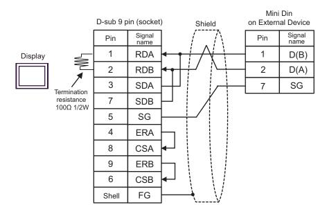
C) When using the online adapter (CA4-ADPONL-01), the connector terminal block conversion adapter (CA3-ADPTRM-01) by Pro-face and your own cable
