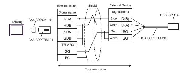
D) When using the online adapter (CA4-ADPONL-01) by Pro-face, your own cable, the Uni-Telway connection cable (TSX SCP CU 4030) and the PCMCIA card for RS485 (TSX SCP 114) by Schneider Electric
