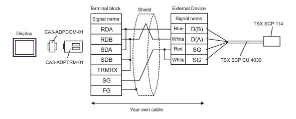
B) When using your own cable, the Uni-Telway connection cable (TSX SCP CU 4030) and the PCMCIA card for RS485 (TSX SCP 114) by Schneider Electric
