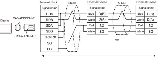
B) When using the accessory box (TSX SCA 50) by Schneider Electric and your own cable
