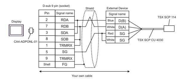
E) When using the COM port conversion adapter (CA3-ADPCOM-01), the connector terminal block conversion adapter (CA3-ADPTRM-01) by Pro-face, the Uni-Telway connection cable (TSX SCP CU 4030) and the PCMCIA card for RS485 (TSX SCP 114) by Schneider Electric
