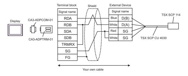
F) When using your own cable, the Uni-Telway connection cable (TSX SCP CU 4030) and the PCMCIA card for RS485 (TSX SCP 114) by Schneider Electric
