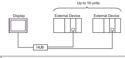
• Connecting multiple Series 90-30 devices requires a V6.50 or higher CPU. Check the version of the CPU in the dialog box displayed by clicking [Online Commands]-[Show Status] from the [Target] menu of the ladder software.
