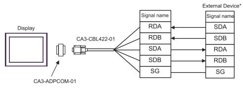
Do not connect the FG terminal of CA3-CBL422-01 to the External Device.
