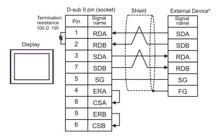
\* Turn On the termination resistance switch of the External Device, and set the operation mode to 3.
