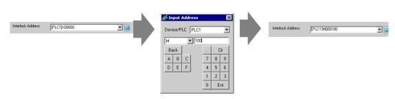
3 Use the [Touch Enable Condition] field to set up a condition that enables touch operations. (For example, select "Enable When Bit is Off" to enable touch operations when the bit is off.)
