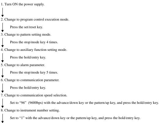
Set to "NOML" (serial communication) with the advance/down key or the pattern/up key, and press the hold/entry key.
