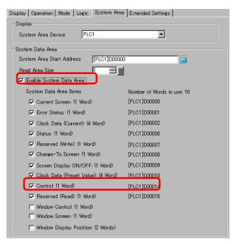
4 If you turn ON Bit 1 in the [Control: (1 Word)] address specified in step 3 while Bit 5 is OFF, the contact to sound an external buzzer turns ON. You can then connect and operate an external power supply and a buzzer or revolving light.
