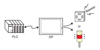
The GP AUX terminal connector can be used for external audio output devices.
