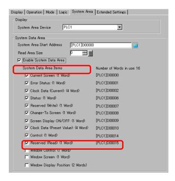
4 If you turn ON Bit 1 in the [Control: (1 Word)] address specified in step 3 while Bit 4 is OFF, the GP main unit buzzer rings.
