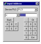
6 Click the icon and select the [Device/PLC] and [Device]. Input an address from the keypad. (For example, M100)
