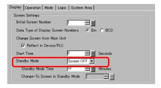
4 In [Standby Mode Time], set the time to wait between the last touch and turning OFF the screen.
