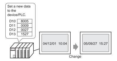
Sets the GP clock data (BCD) from a device/PLC.
