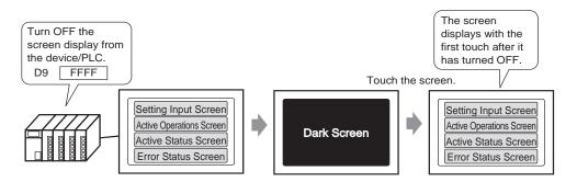
Turns OFF the GP screen display from a device/PLC.
