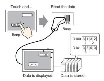
The code data read from a two-dimensional code reader can be stored in a device/PLC's device address through data display parts or can be stored in the GP's internal device address.
