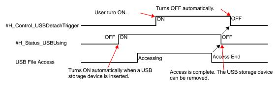
When #H\_Status\_USBUsing is OFF, you cannot access the USB storage device. Remove the USB storage device and insert again.
