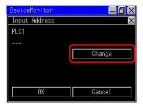
5 Input the address you want to display and touch [ENT]. The screens will be switched. Touch [OK] to display the input address on the random monitor screen.
