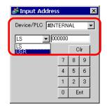
The GP's internal device [#INTERNAL], has two structured areas: the [LS] area and the [USR] are (shown below).
