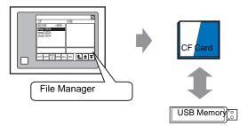
1 From the [Parts (P)] menu, point to [Special Data Display (P)] and select [File Manager (M)]. Place File Manager on the screen.
