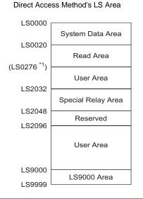
MPORTANT • Do not set addresses for Parts which span the System Data Area and Read Area, or the Read Area and User Area.
