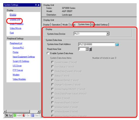
2 Allot the addresses in the device/PLC you will communicate with. In [System Area Device], select the device/PLC where you will allot addresses and set the start address of an area that has 16 Words or more of continuous addresses in [System Area Start Address].
