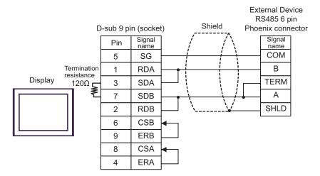
C) When using the online adapter (CA4-ADPONL-01), the connector terminal block conversion adapter (CA3-ADPTRM-01) by Pro-face, and your own cable
