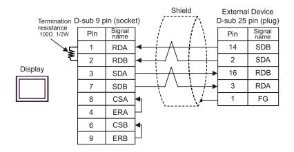
C) When using the online adapter (CA4-ADPONL-01), the terminal block conversion adapter (CA3-ADPTRM-01) by Pro-face and your own cable
