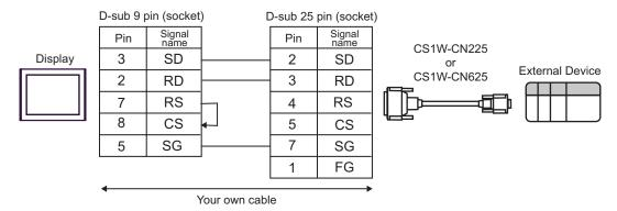
B) When using CS1W-CN226 (2m) or CS1W-CN626 (6m) by OMRON Corporation or your own cable
