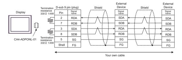
• In order to improve noise resistance characteristics, please use a twist pair whole shield cable as a transmission cable and ground the shield line.
