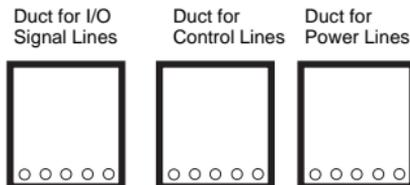
If different wires must be placed in the same duct, separate them using grounded dividers.
