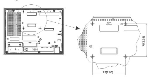
1) Attach one screw to the Display's rear face. The torque should be 0.5Nm to 0.6Nm.
