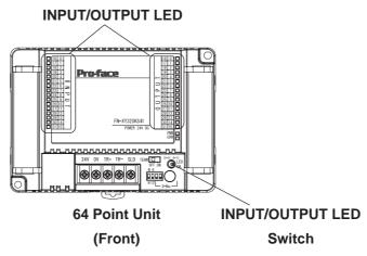
When the INPUT/OUTPUT LED Changeover Switch is set to [0-15], as shown below, the INPUT/OUTPUT LEDs display [INPUT0] to [INPUT15], and from [OUTPUT0] to [OUTPUT15].
