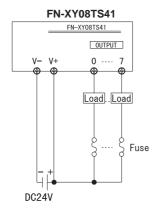
When attaching two (2) Transistor Ouput units (FN-XY08TS41/FN-Y16SC41/FN-Y16SK41/FN-XY16SK41/FN-XY16SC41/FN-XY32SKS41) with the same Common line, be sure to use the wiring shown below.
