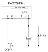
When using the Transistor output unit, (FN-XY08TS41/FN-Y16SC41/FN-Y16SK41/FN-XY16SK41/FN-XY16SC41/FN-XY32SKS41), be sure to connect a Reverse Start Power Absorbing Diode to both ends of the load.
