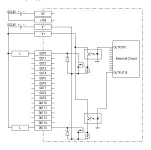
The I/O unit's power supply should be separated from **Note:** The I/O unit's power supply should be set of the sensor's power supply to prevent the unit from being affected by external noise.
